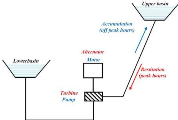
**Fig.1 The process of a pumped hydro storage [10].**
