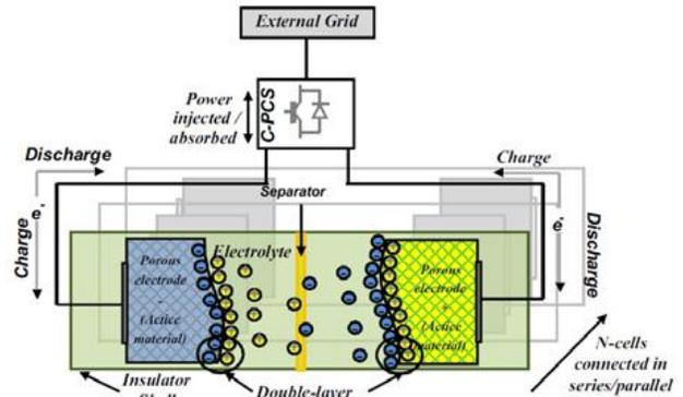
**Fig.2 The capacitor storage system [10].**
