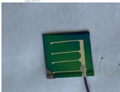
**Fig. 2 External view of the PV sample.**
