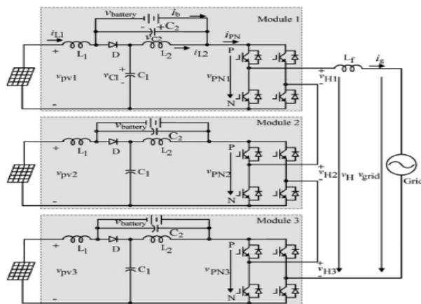
Fig. 1. PV based seven level QUASI-Z-SOURCE Inverter
