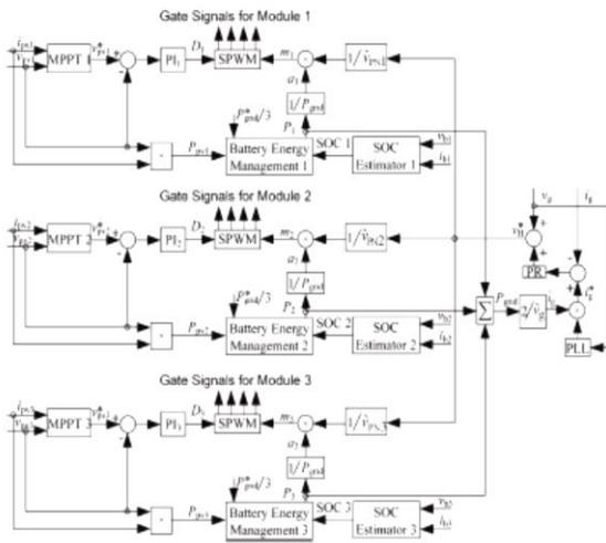
**Fig.5. Control scheme for the proposed system.**
