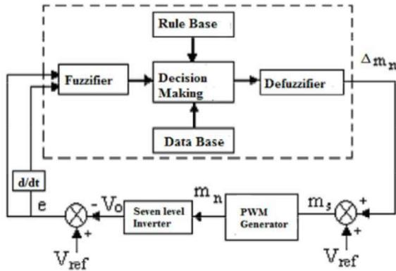
*Fig7 : Fuzzy logic control scheme for Quasi Z-source*
