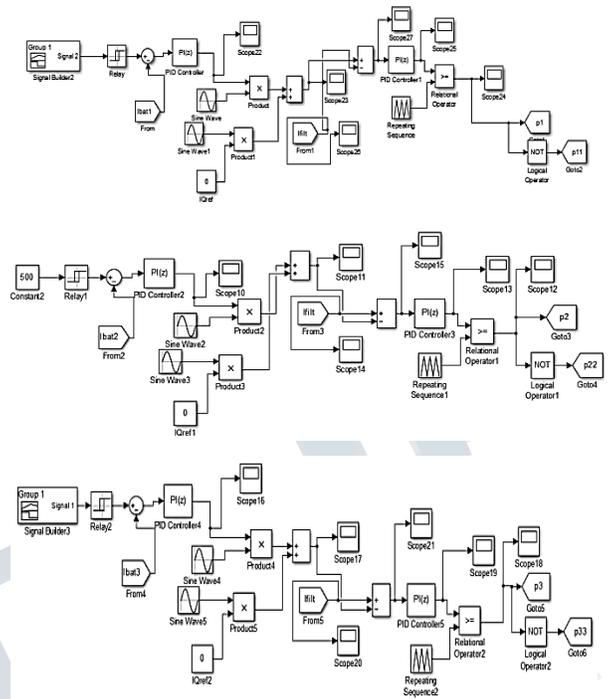
*Fig.8. Control circuit without fuzzy controller.*
