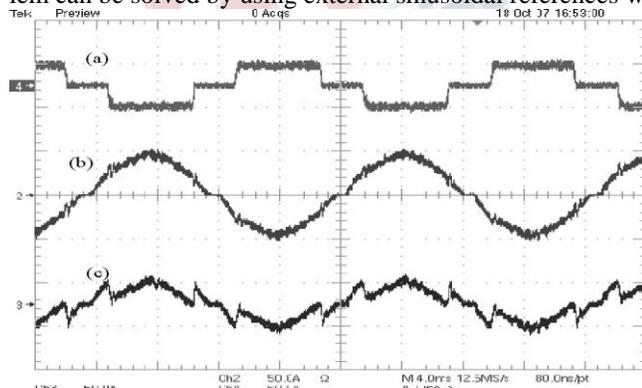
**Fig. 14. Experimental waveforms. (a) Single-switch boost rectifier current. (b) Line current. (c) PWM unidirectional rectifier current**
