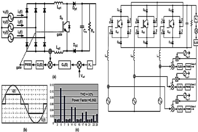
**Fig. 2. (a) Single-switch three-phase boost rectifier power stage. (b) Waveform of the input voltage and current. (c) Harmonic content of the input current.**
