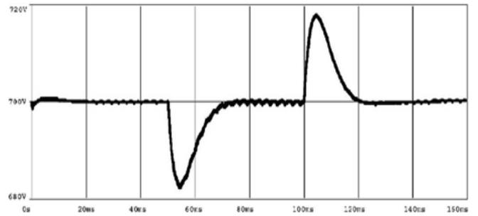
**Fig. 11. Output voltage transient response to a load change**
