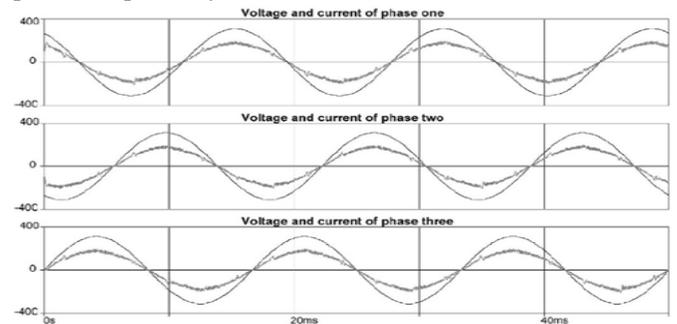
**Fig. 8. Input voltages and input currents (scaled up 4x) of the simulation**
