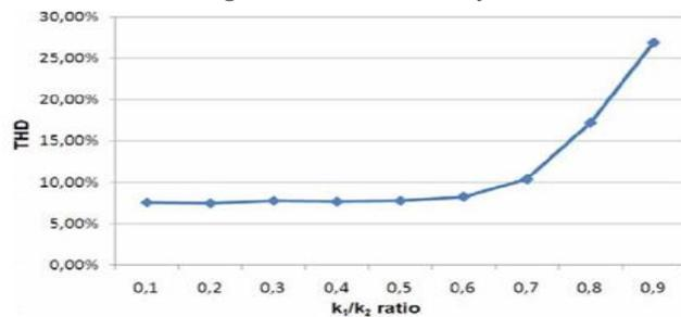
**Fig. 18. THD versus ratio of  $k_1$  and  $k_2$ .**
