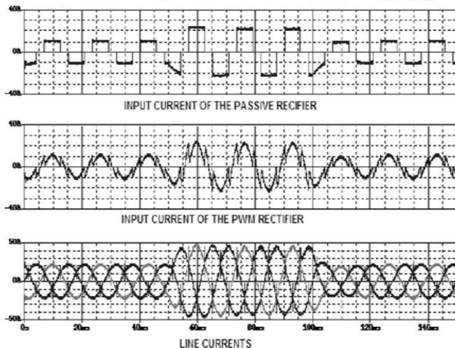
**Fig. 10. Load step response generated by simulation.**
