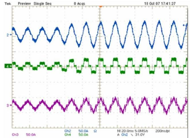
**Fig. 15. Experimental waveforms to a load step. (a) Line current. (b) Single-switch boost rectifier current. (c) PWM unidirectional rectifier current.**
