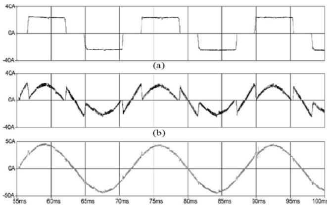
**Fig. 9. Simulation results. (a) Current at the input of the passive rectifier. (b) Current at the input of the active rectifier. (c) Total current drawn from the source**
