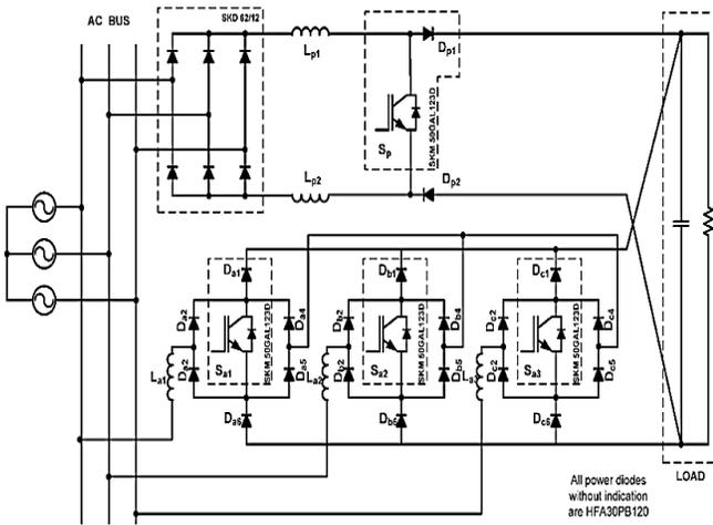
**Fig. 1. Hybrid three-phase high -power-factor rectifier. The traditional single-switch three-phase boost rectifier and the three-phase boost unidirectional rectifier connected in parallel.**
