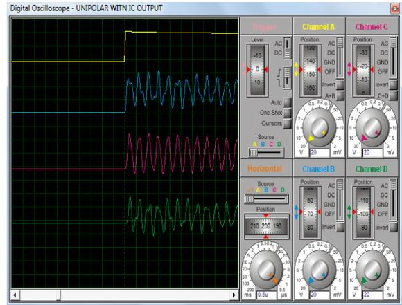
**Fig.5 Intercoil Voltage Distribution-Unipolar Pulse**
