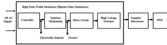
Fig.2 Block Diagram
