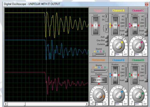
**Fig.6 Interturn Voltage Distribution-Unipolar Pulse**
