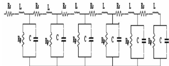
Fig.1 Winding Model
