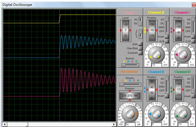
**Fig.8 Interturn Voltage Distribution-Bipolar Pulse**
