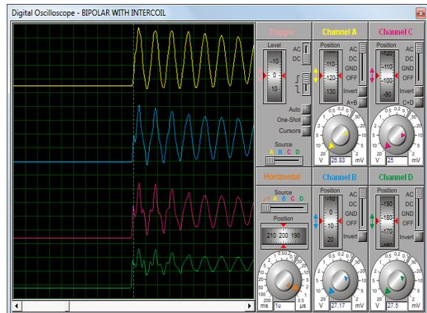
**Fig.7 Intercoil Voltage Distribution-Bipolar Pulse**
