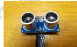
**Fig 5.1 Ultrasonic Sensor**
