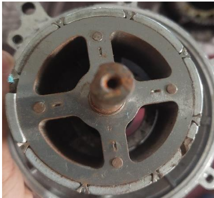
Fig. 4 Rotor of a BLDC Motor
