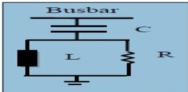
1. Determining the capacitor size  $Q_c$  in MVAR, say the reactive power requirement of the harmonic source.
