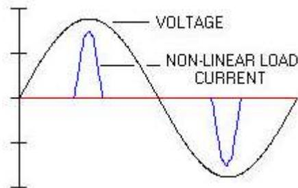
Fig[1] Waveform with non linear load
