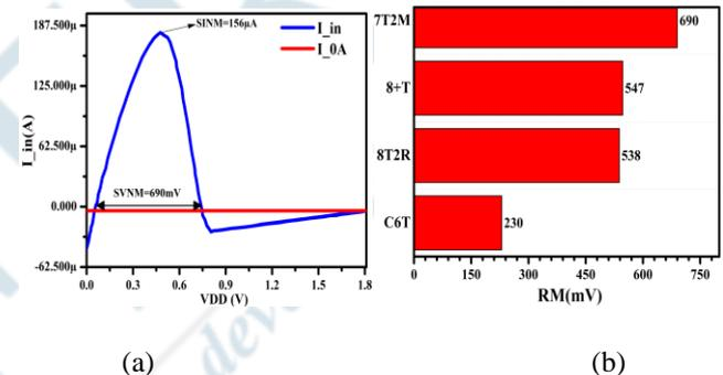
Figure 6: (a) N-curve for RM calculation (b) Read margin comparison of various SRAM cells at VDD=1.8V.
