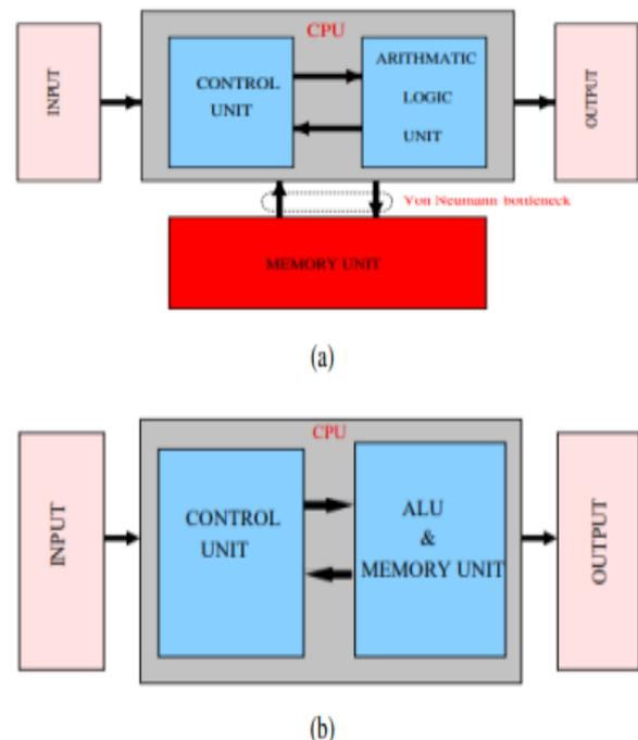
**Figure 1:** a) The conventional computing system with an illustration of the Von-Neumann bottleneck. b) The IMC system with an illustration of computational memory and ALU.
