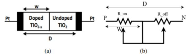
Figure 2: (a) The Device structure of Memristor. (b) The equivalent circuit of Memristor.
