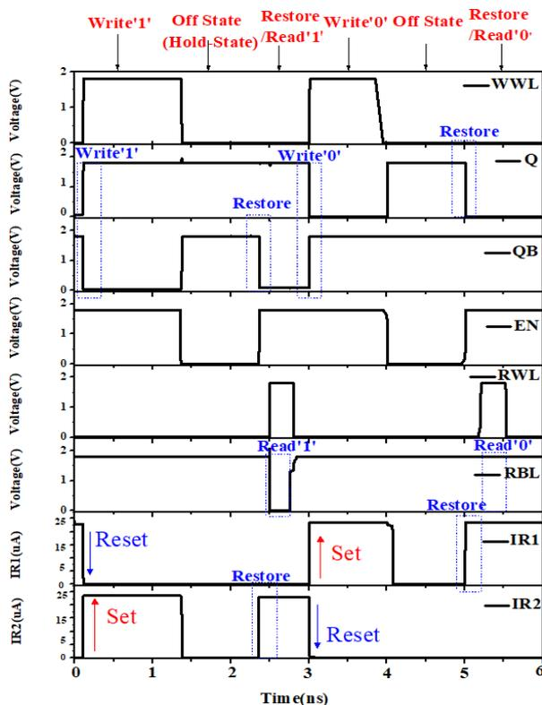
Figure 5: Timing waveform of 7T2M NvSRAM array for write, store/off state and self-restore/read operation.
