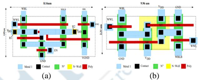
Figure 8: Thin cell Layout of (a) 7T2M NvSRAM. (b) C6T
