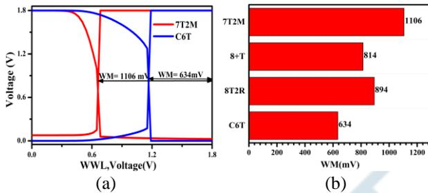
Figure 7: (a) WM calculation of proposed 7T2M NvSRAM. (b) WSNM comparison of various bit-cells at VDD = 1.8V.
