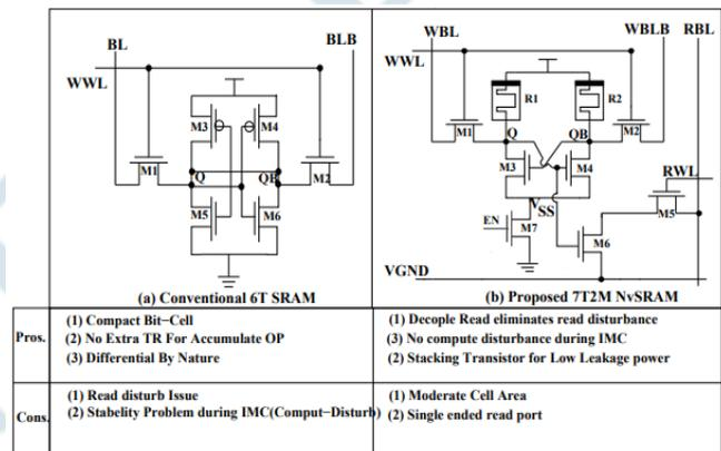
Figure 3: Comparison of C6T, and Proposed 7T2M NvSRAM.
