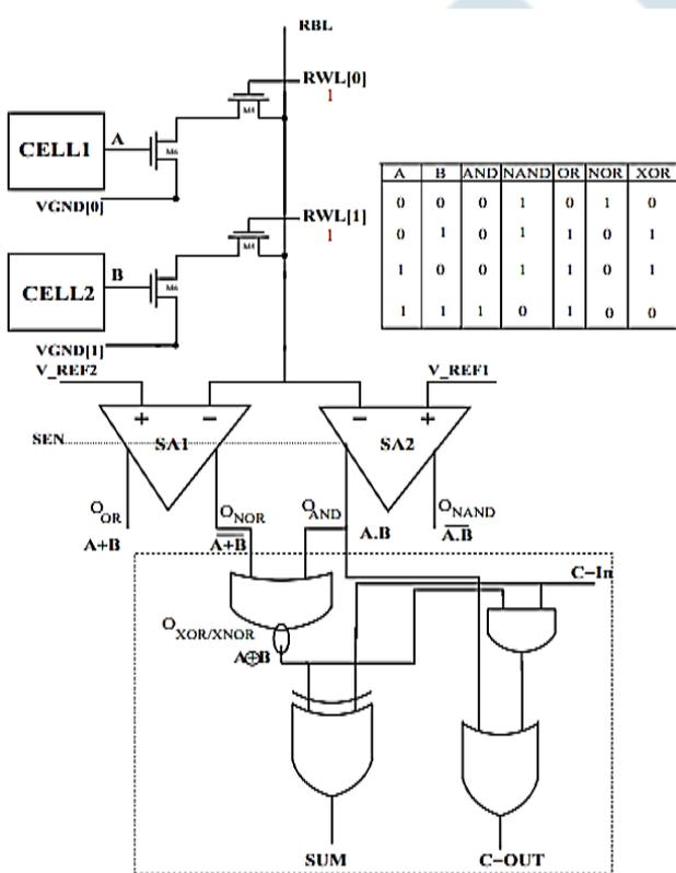
Figure 9: The schematic of circuit for performing IMBC operation.
