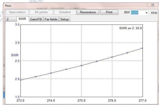
Fig. 5: VSWR simulated output
