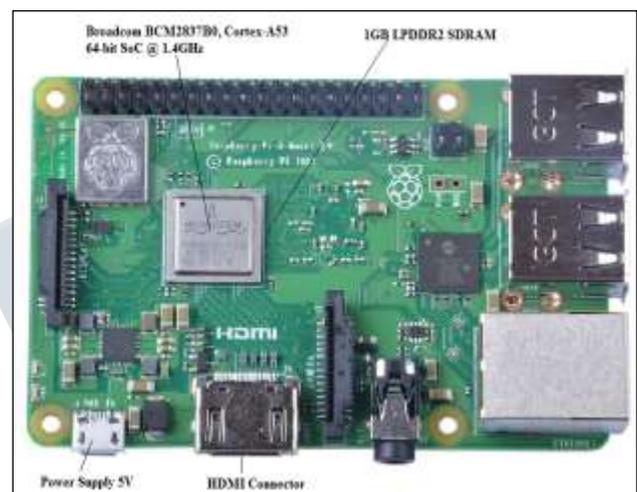
**Fig.3. Raspberry pi 3 B+ Model**
