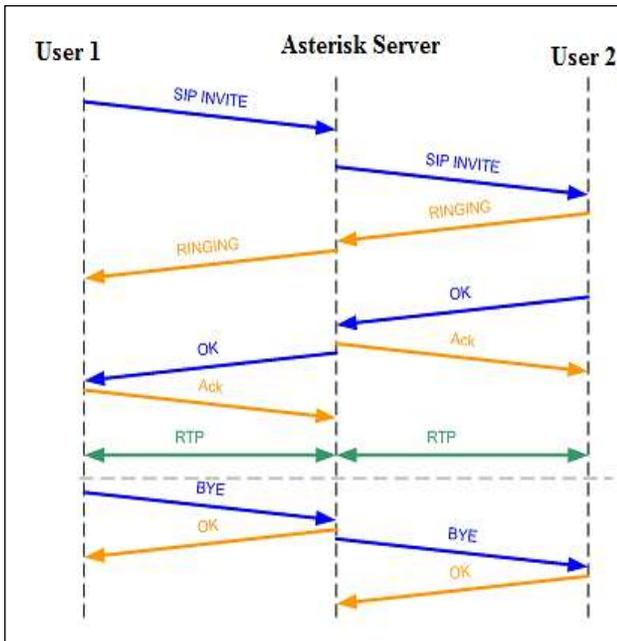
**Fig.5. The connection establishing method from user extension to asterisk server**
