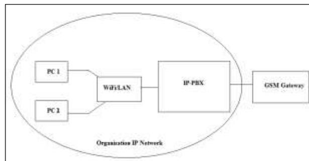
**Fig.1. IPPBX System architecture with GSM gateway**
