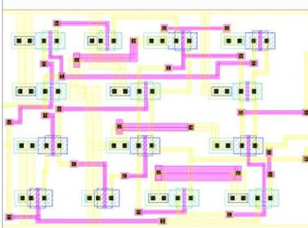
**Fig. 11** Circuit layout of HFA- 14T-2
