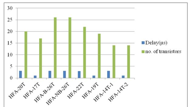
**Fig. 13 simulation results: No. of transistors vs. delay**
