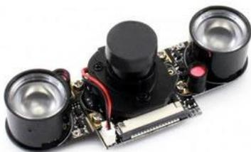
**Figure 3: Stereoscopic camera (5MP OV5647)**
