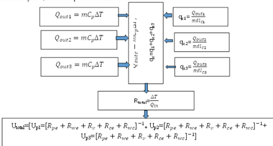
Figure 5 Heat Transfer, heat flux and Overall Heat Transfer Coefficient calculation procedure of PCM heat pipe
