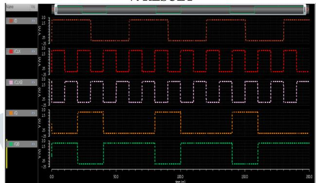
*Figure 3. Output waveform of D flip-flop*
