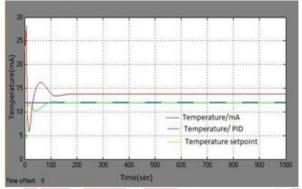
Figure.4 Simulation graph for Temperature control
