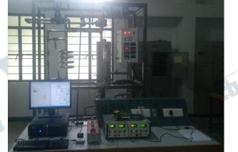
Figure.7 Experimental setup of CSTH Process
