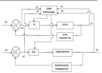
Figure.1 Automatic gain scheduling Controller Design for CSTH Process
