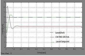
Figure.3 Simulation graph for Level control
