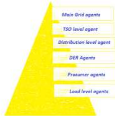
Fig. 1. Control Architecture of Power Grid
