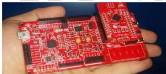
Fig 2: PSoC Pioneer Board [8].
