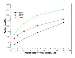
Fig. 10 PLR vs Packet rate
