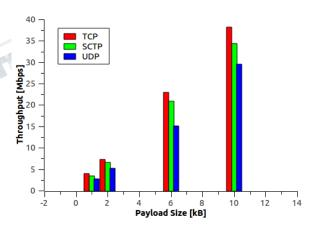
Fig. 2: Throughput vs payload size in LAN
