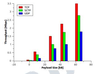
Fig. 6: Throughput vs payload size in WAN
