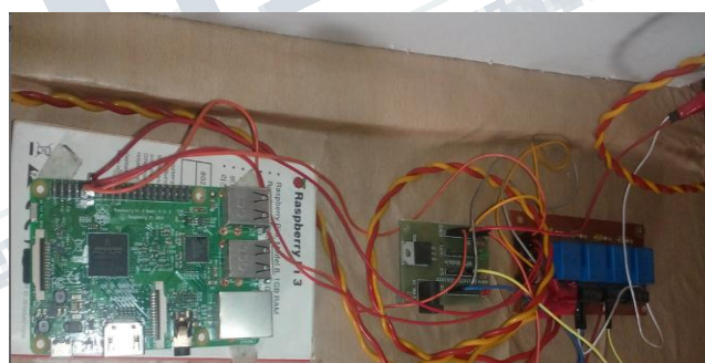
Image 6.1. Raspberry pi connected with Relay.
