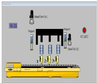
Fig. 2 Three LPG cylinders entering the sealing unit
