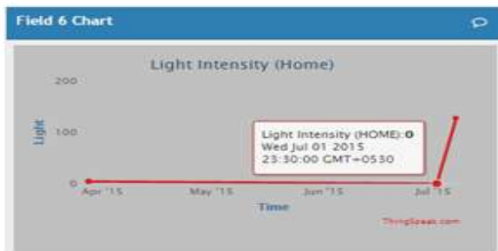
Fig. 6c Light intensity result on ThingSpeak API
