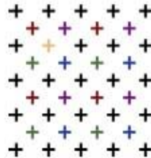
Fig.4. Position of the center of pixels in the original image u in black, in the four sub-images \tilde{u}_1 in red, \tilde{u}_2 in purple, \tilde{u}_3 in green and \tilde{u}_4 in blue.
