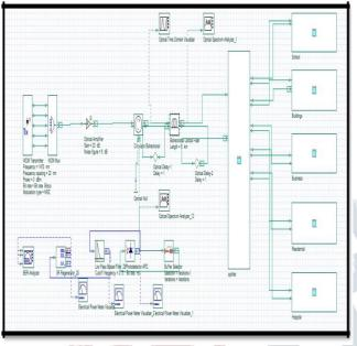
Fig.1. Design of WDM-PON
