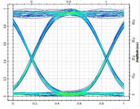
Fig.7. Eye diagram for Residential block
