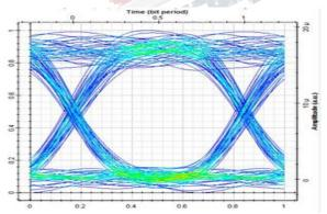
Fig.9. Eye diagram for upstream transmission
