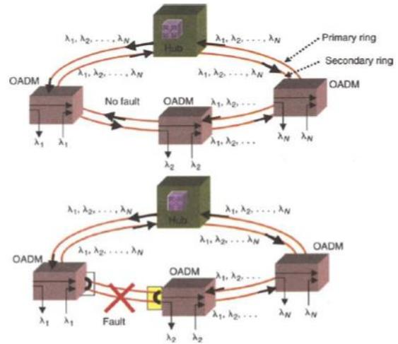
Figure 3: DWDM ring network topology to detect faults
