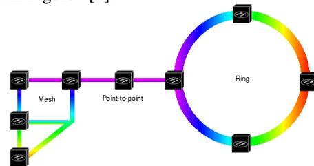
Figure 4: Mesh, Point-to-Point, and Ring Architectures
