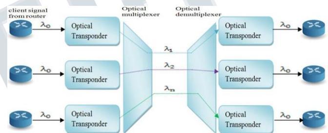
**Figure 1: A point-to-point DWDM network**
