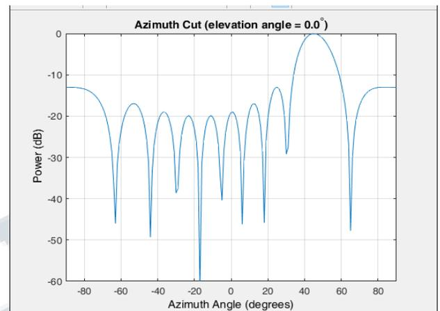
**Fig3: Plot array response with weighting**
