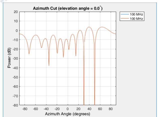
**Fig4: Plot array response with interference**
