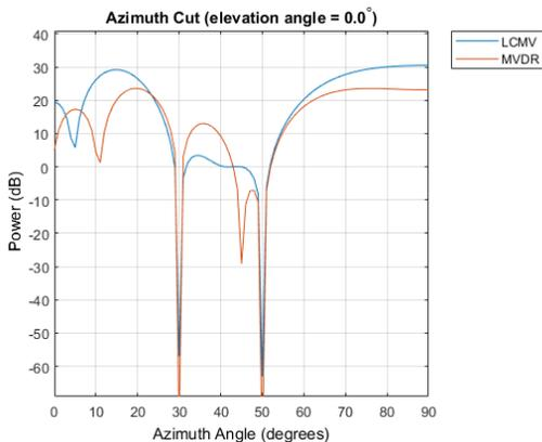
**Fig6: Beamformer response with interference**
