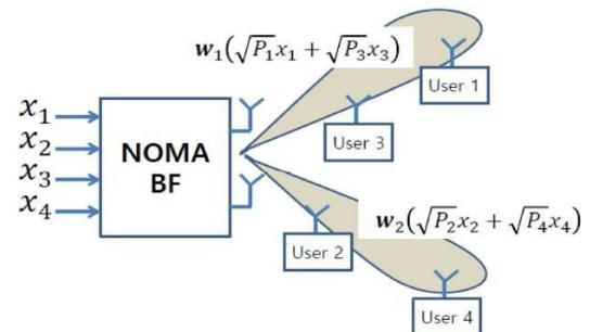
*Fig1: An illustration of NOMA with beam forming.*
