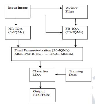
Fig.1. Block diagram of proposed Liveness Detection method
