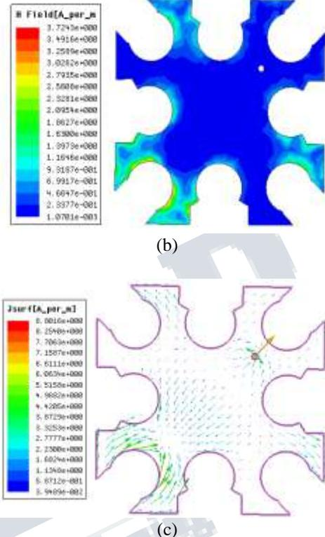
**Fig.8. (a) E Field (b) H Field (c) J Field distributions of the Proposed Antenna**
