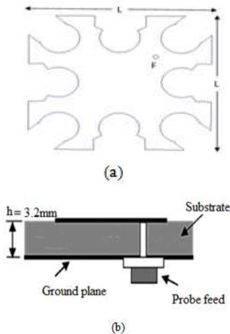
**Fig.1. (a) Proposed Antenna (b) Feed Position.**
