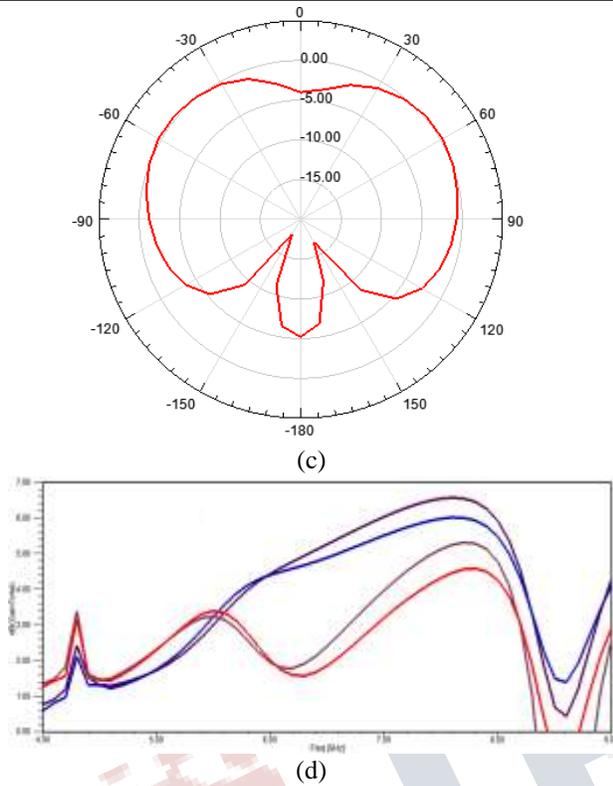
**Fig.7. (a) Return loss (b) VSWR (c) Radiation Pattern (d) Gain of the proposed antenna**
