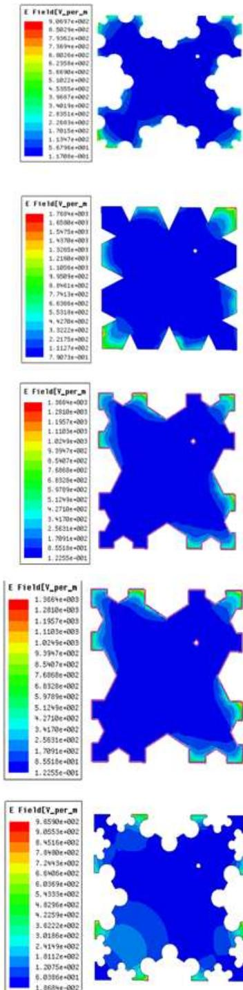
**Fig.4. E Field Distribution of the Four Designed Antennas**
