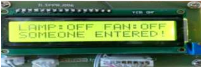
Fig -8: Status of home security displayed on LCD
