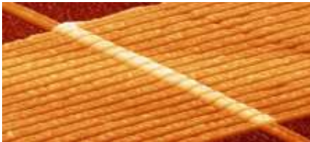
Electron photo of 17 titanium dioxide MEMRISTORS
