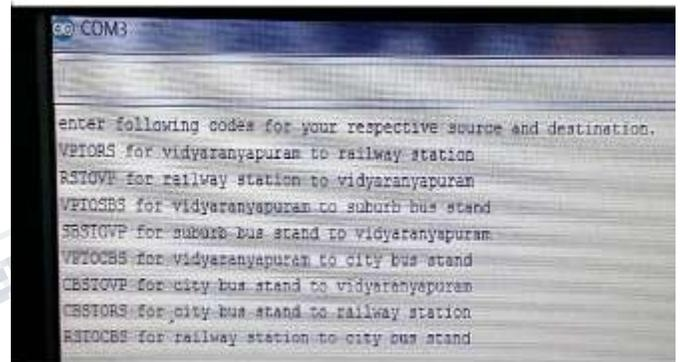
*Fig 4: After uploading the program to the Arduino Duemilanove, the codes to be entered is listed for calculation.*
