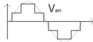
Fig.3: Waveform of a five level multilevel inverter
