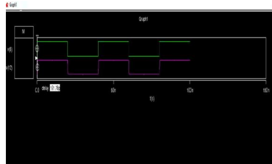
Fig 4(a): Simulation results showing Delay in previous design system (MHLFF)
