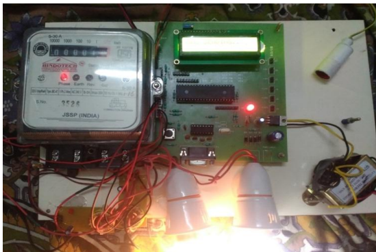
Fig 9: Hardware implementation of integrated energy meter
