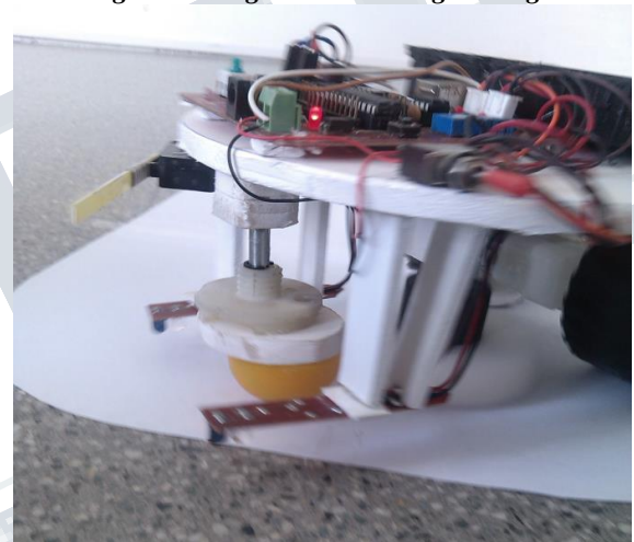
Fig. 3.3 Swing robot changing direction to avoid the edge
