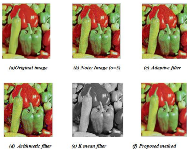
Figure.4 Restoration Results of Pepper image corrupted with a noise standard deviation ( \sigma=5 ) by various filters
