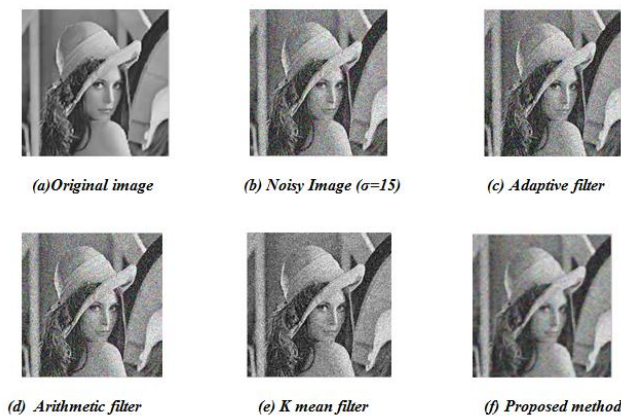
Figure.3 Restoration Results of Lena image corrupted with a noise standard deviation ( \sigma=15 ) by various filters
