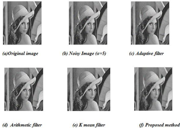
Figure.2 Restoration Results of Lena image corrupted with a noise standard deviation ( \sigma=5 ) by various filter
