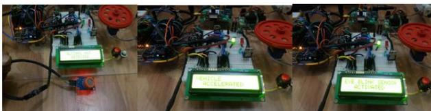
Once the vehicle starts to accelerated the eye blink sensor is activated, this sensor detects if the driver has slept or not while driving.
