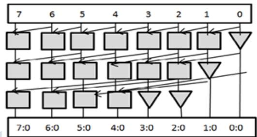
**Fig.5.8-Bit Kogge Stone Adder**
