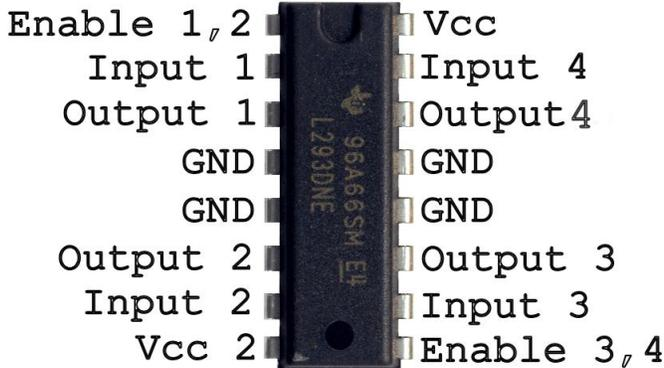
The Device is a monolithic integrated high voltage, high current four channel driver designed to accept standard DTL or TTL logic levels and drive inductive loads (such as relays solenoids, DC and stepping motors) and switching power transistors.
