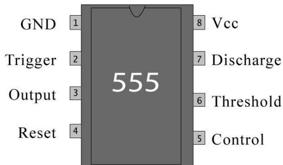
**GND:** Ground reference voltage, low level (0 V).
