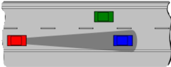
According to this distance the micro controller controls the speed of motor using the PWM technique to control the speed of motors. If the distance between cars is more, then microcontroller will not limit the cruising speed. As the distance between cars decreases, microcontroller will start to reduce the cruising speed. If distance reduces to very small value then microcontroller will stop the motors and hence the car will stop.
