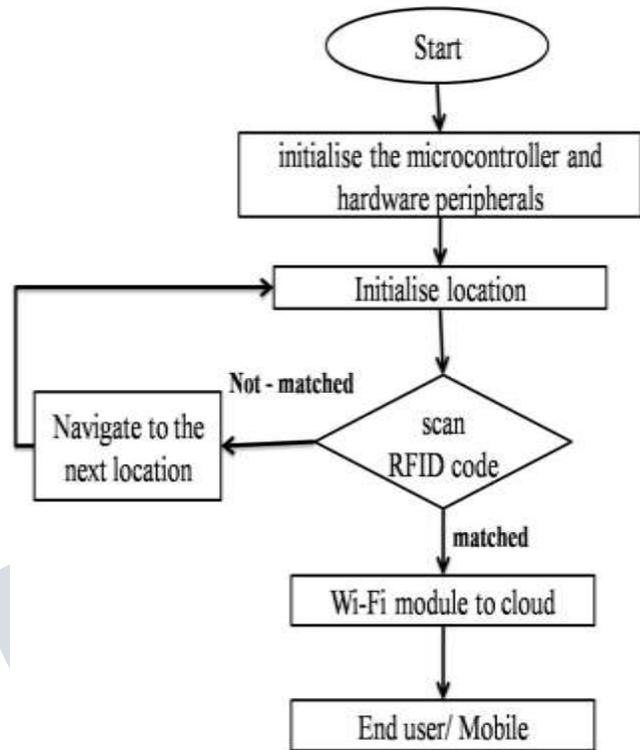
**Figure 4** Flowchart describing person identification using RFID tag
