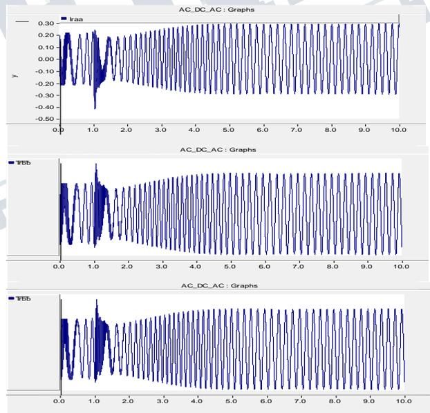
Fig 1 Turbine rotor current during speed variation
