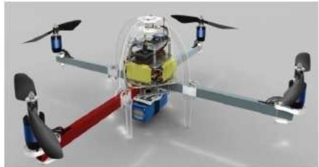
The design drives four rotors using the Ardupilot board. No tail rotor is needed and control was obtained by varying the thrust between rotors.
