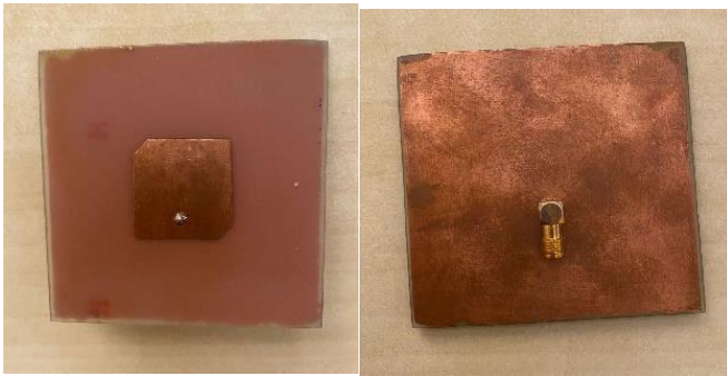
Fig: Fabricated Microstrip Patch Antenna
