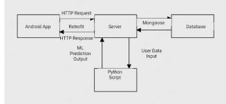
Fig IV.1 System Architecture
