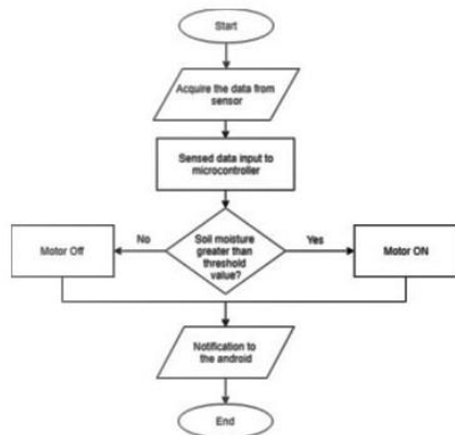
Fig. 2. Flow chart of Smart Farm Irrigation System
