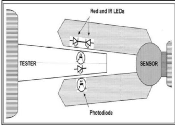
**Fig. 2.1. Working of SpO2 Sensor**
