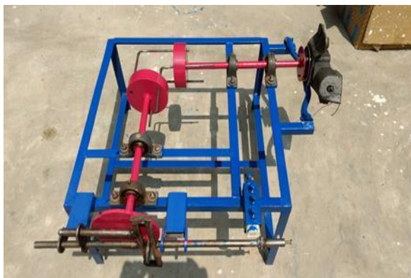
Fig-7: Gearless power transmission for skew shafts
