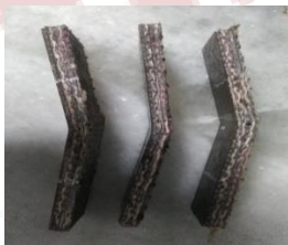
Fig. 22. Flexural test Specimen of Banana-Jute composite after testing
