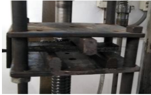
Fig. 18. Test set up for three point bending tests
