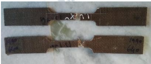
Fig. 11. Tensile Samples of Specimen A after testing
