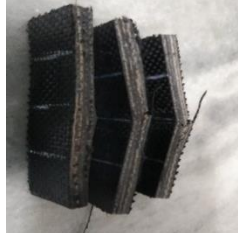
Fig. 23. Flexural test Specimen of Carbon Banana-Jute composite after testing
