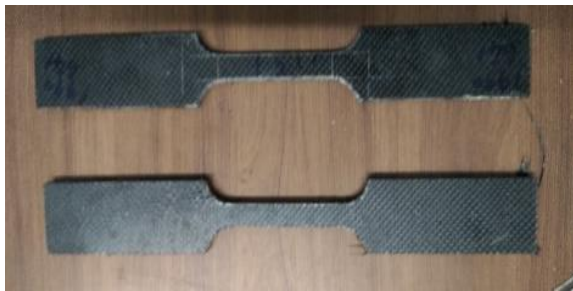
Fig. 14. Tensile Samples of Specimen B before testing
