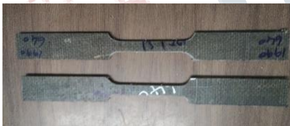
Fig. 10. Tensile Samples of Specimen A before testing
