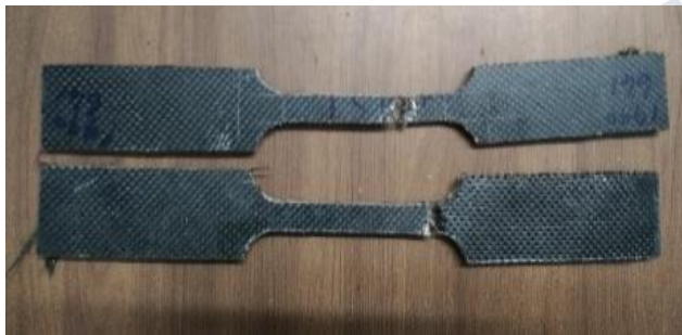
Fig. 15. Tensile Samples of Specimen B after testing
