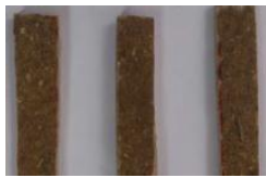
Fig. 20. Flexural test Specimen of Banana-Jute Composite (Specimen A)
