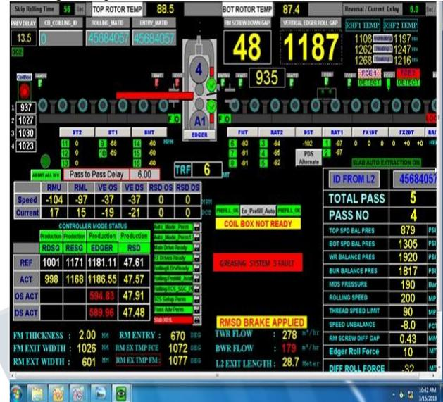
Fig.6- Fault Output in Human Machine Interface
