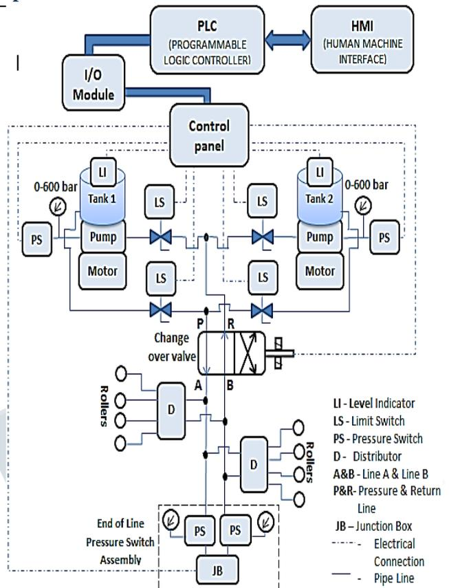
**Fig.1- Proposed Automatic Dual Line Lubrication System**
