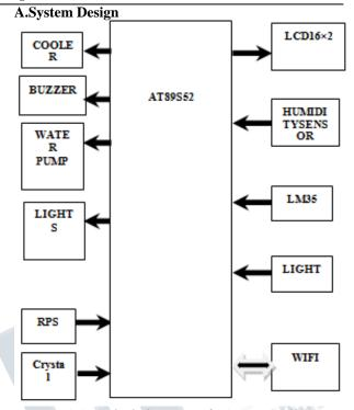
Fig3.1:Block diagram of microcontroller
